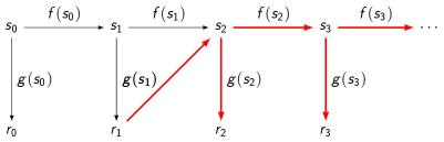
XXX's mission: Predict the "random" output bits. Create protocols that directly output  $r_n$  for some reason. Design f, g with back door from  $r_n$  to  $s_{n+1}$ : i.e., get f(s) from g(s).
