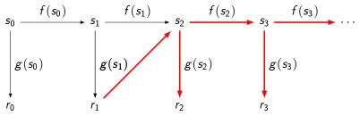
XXX's mission: Predict the "random" output bits. Create protocols that directly output  $r_n$  for some reason. Design f, g with back door from  $r_n$  to  $s_{n+1}$ : i.e., get f(s) from g(s). Standardize this design of f, g.
