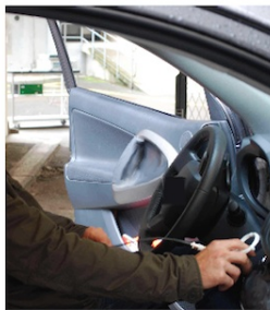
(b) Starting the engine using the relay.
