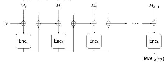
This picture shows how  $\mathsf{MAC}_k(m)$  is computed. The input are the key k and message  $m = (M_0, M_1, M_2, \dots, M_{\ell-1})$ . The output are the chosen IV and  $\mathsf{MAC}_k(m)$ .
