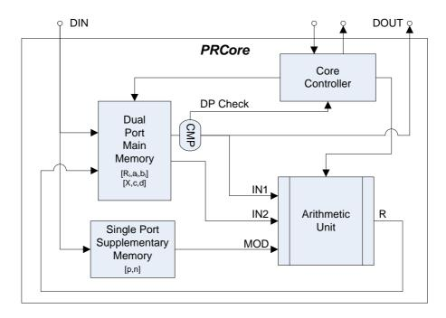
Figure 4: Core layer of an FPGA-based point processor
