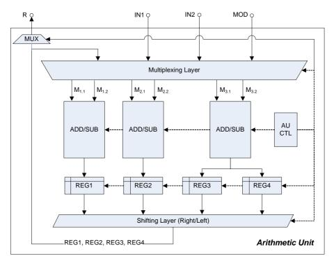
Figure 5: Arithmetic layer of an FPGA-based point processor
