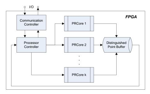
Figure 3: Top layer of an FPGA-based point processor
